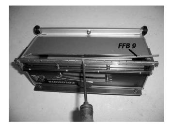
3) Blade out. \*\*Notice slight bends at each end of blade. When installing new blade, it is important to bend each end slightly. This creates tension that keeps blade in holder.
