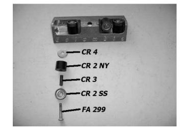
3) Roller parts removed from head casting.
