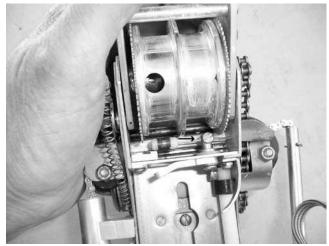
Use small screwdriver to push roller (CT 16) and ratchet rod (CT 15) in direction shown. 4) Turn adjusting lever outward until brake roller clears wheel.
