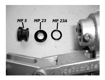
Remove hex bolt that holds piston cup assembly to shaft. Use 1/2" ratchet or wrench.
