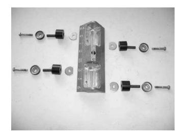
4) New roller assembly. The Columbia corner roller uses components for the easiest, most reliable possible operation. The main nylatron part of the roller makes the operation easy. The steel finishing part provides a crisp, sharp bedding of the corner tape and longterm durability.
