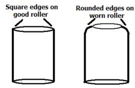
When the bearing sleeves become worn as shown, the roller may not track square in the corner. If your sleeves look like the worn version, they should be replaced. When rollers become noticeably worn as shown, they should be replaced.
