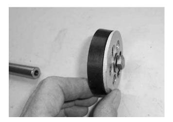
16) Second view of piston cup assembly with bolt and washer in place.
