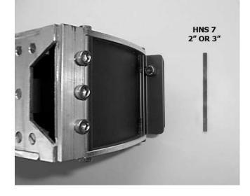
Blade should be set .002" or "thumbnail click" higher than body shoe where the blade and body meet.
