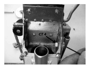
9) Use small screwdriver to push old CT 5 nyliner out of insert bushing.
