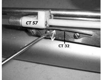
Set feed needle so the sharp point goes 1/16" through feed guide as shown in picture 2 and diagram. Tighten screw.
