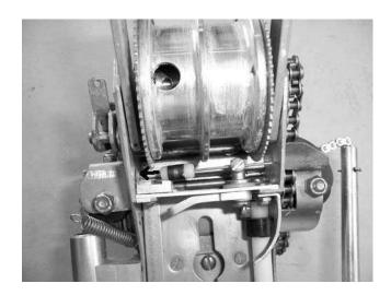
8) Use end of small screwdriver to push rod and roller into position. The roller should have just enough clearance (approximately 1/64") from the side plate so that lever adjusts roller freely. Tighten set screw and adjust tension as desired.
