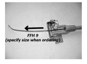
10) One end of the new strap has a larger hole. Bend slightly as shown- this will give the braking a return spring action.
