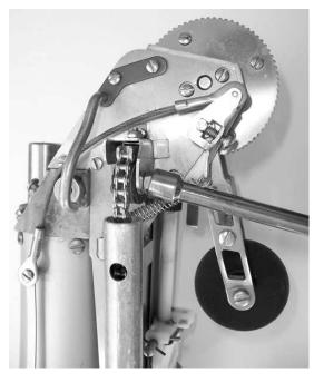
7) Remove screw that attaches roller and bushing to bracket. Remove old roller from screw and bushing.
