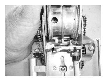
5) Use needle nose pliers to remove roller and rod.
