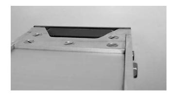
4) To replace pivot parts, remove lock nut FA 271 with 3/8" nut driver or wrench and medium blade screwdriver.
