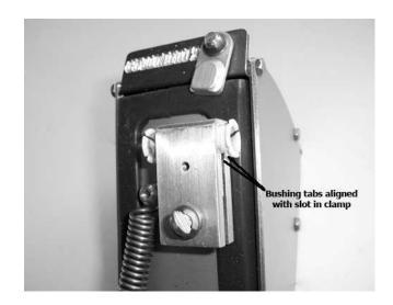
7) Insert handle roll pin with screw into bushings in clamp.
