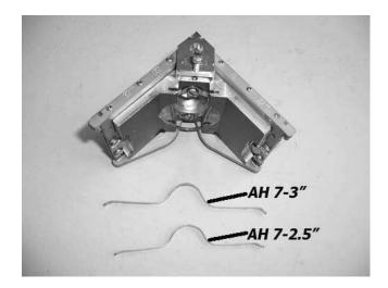
3) Remove retainer clips that hold frames together. 5/64" hex key fits these setscrews FA #258. Start with bottom clip AH 9
