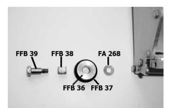
15) Installing new o-rings on wheels can make your box run more smoothly on finish seams. Use pick or small screwdriver to remove old o-ring.
