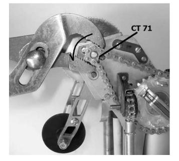
2) Use 5/64" hex key to remove set screw that holds drive drum to drive shaft.
