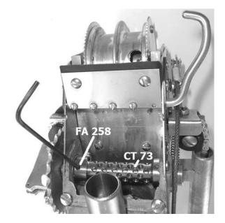
7) Note order of parts as this will be important when re-assembling. Also note there are two CT 76 nylatron washersone goes between the large gear and head casting and the other goes between the cable drum and head bushing inside the head.
