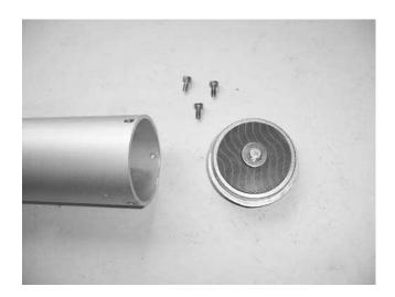
26) Remove wing nut and screen (MP 24) from valve assembly.
