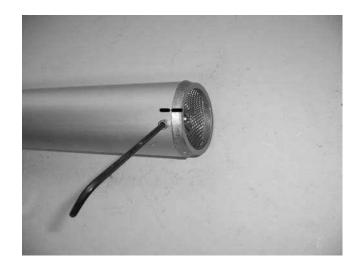
34) Re-install pump cylinder onto pump head and clamp latches.
