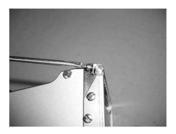
Use screwdriver to carefully lift old blade (FFB 9) out of blade holder. Back off adjusting screw so it is flush with bottom of blade holder slot.
