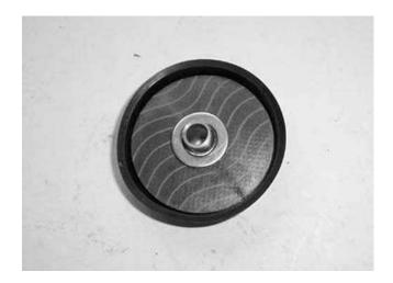
14) Put on large retainer assembly. The locator and sleeve will align everything properly.
