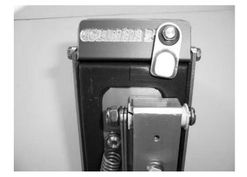
\*\* Many people do not use the spring and the nail spotter will work without it. HOWEVER, with the spring on, it makes it easier to pull nail spotter cleanly away from wall or ceiling without leaving a tail of mud.
