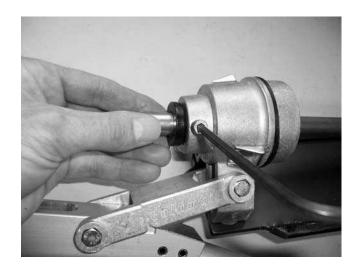
23) Attach piston shaft to handle with handle pin.
