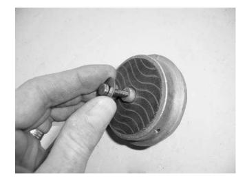
31) Hold hex bolt with 5/16" wrench or nut driver and install lock nut with 3/8" nut driver.
