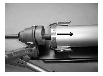
3) Pump cylinder off. Remove piston shaft assembly from pump head.
