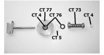
8) Use hex key to push old CT 4 nyliner out of head bushing. Replace with new CT 4.
