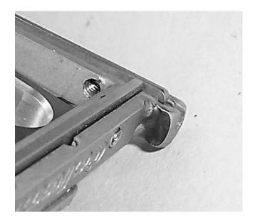
18) Side blade and top blade set properly. This will allow your angle head to do a nice, consistent finish in the corners.
