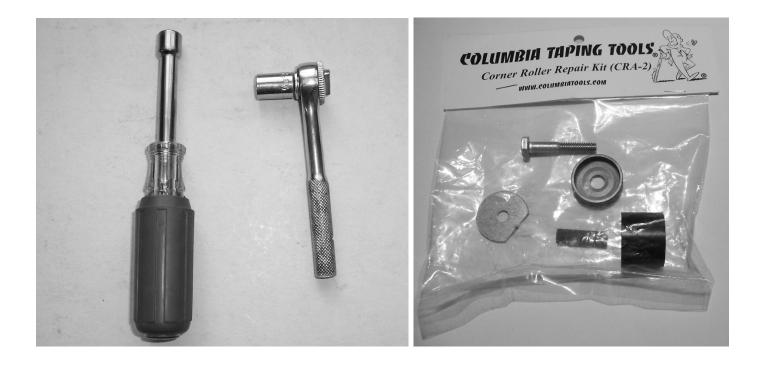
1) Use 7/16" wrench on nut driver to remove hex bolt that holds roller assembly to roller head casting.
