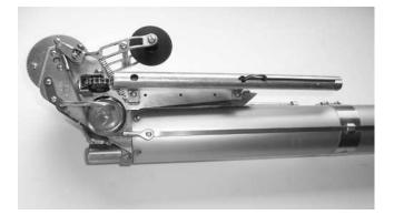
Use small flat blade screwdriver to loosen screw holding cutter blade. <sup>1</sup>/<sub>2</sub> to <sup>3</sup>/<sub>4</sub> turn is plenty- this screw does not need to be removed!
