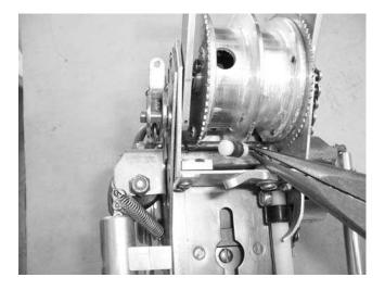
6) Brake roller and ratchet rod out. Put new roller and ratchet rod in holder and turn lever inwards until it looks like next picture.
