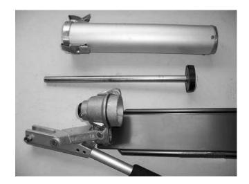
5) Loosen two screws that hold head bushing. Remove bushing, seal and o-ring.
