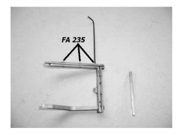
9) Side blade, AH 4 and top blade AH 3 out of frame.
