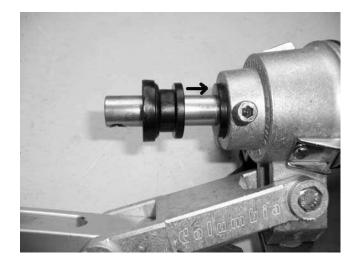
22) Tighten bolts that hold shaft guide in place.
