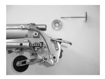
6) Use 5/64" hex key to remove set screw FA 258 from cable drum.
