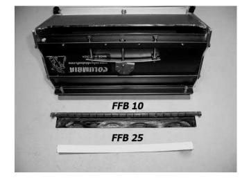
Start new blade bar assembly and gasket holder as shown, working from one end to the other. Gasket holder has slight bend that creates tension. Work carefully into slot.
