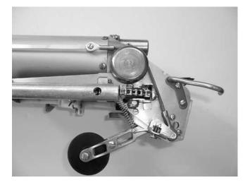
5) Remove pulley and shaft.
