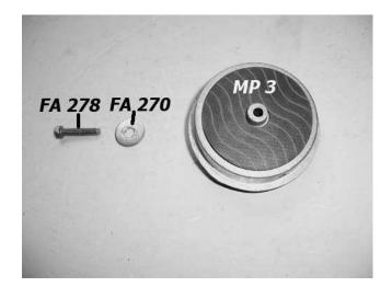
30) Install hex bolt and washer into valve flange.
