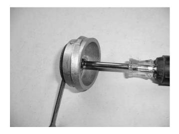
32) Put good screen in valve casting, install wing nut and tighten.
