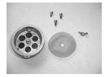
27) Use 5/16" wrench or nut driver to hold bolt on flapper valve side and 3/8" nut driver or wrench to remove lock nut on screen side.
