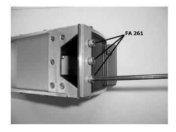
Remove old blade (HNS 7) and check for wear. A sign of wear is a shiny area on blade about 1/4" from either end. If the blade is only worn on one side, it's OK to turn it over and use the opposite finishing side. When ordering replacement blade(s), specify either 2" or 3" HNS 7.
