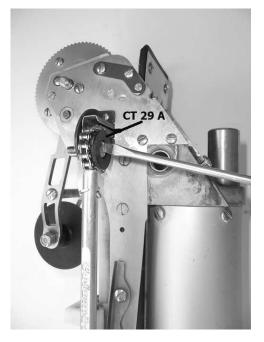
4) Replace with new roller CT 29A and attach roller, bushing and bolt to bracket.
