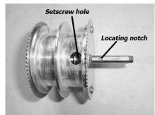
Re-install drive drum on tape Tighten set screw
