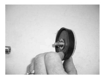
17) Install piston cup assembly to piston shaft and tighten bolt. (Reverse of step 7)
