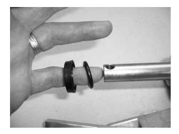
19) Slide seal and o-ring over shaft.
