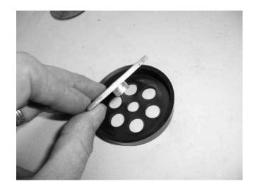
10) Insert sleeve into center of backing washer/ piston cup.
