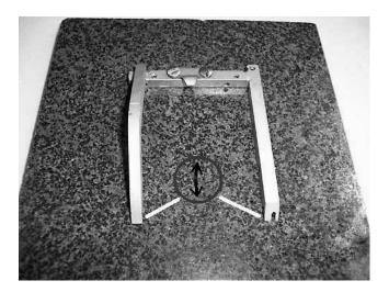
11) Remove set screw that holds retainer spring AH 6.
