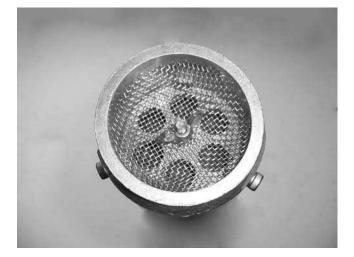
33) Refer to your alignment marks on pump cylinder and valve casting. Install valve casting with three screws and tighten.
