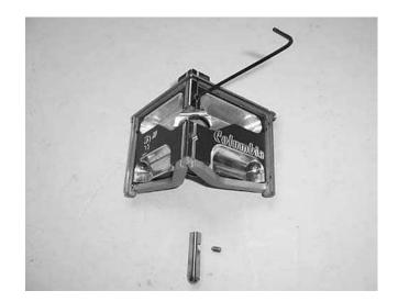
5) Clips off and frames removed from head casting.
