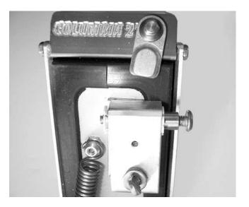
8) Attach connector assembly to clamp with roll pin seated into connector slot before tightening.
