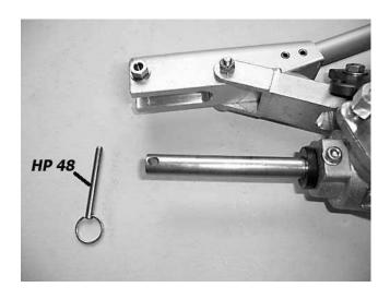
2) Release latch clamps and remove pump cylinder.
