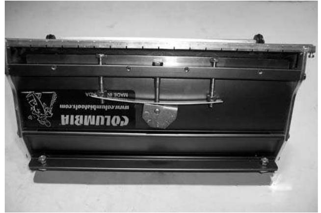
11) Install new retainer clip as shown.
