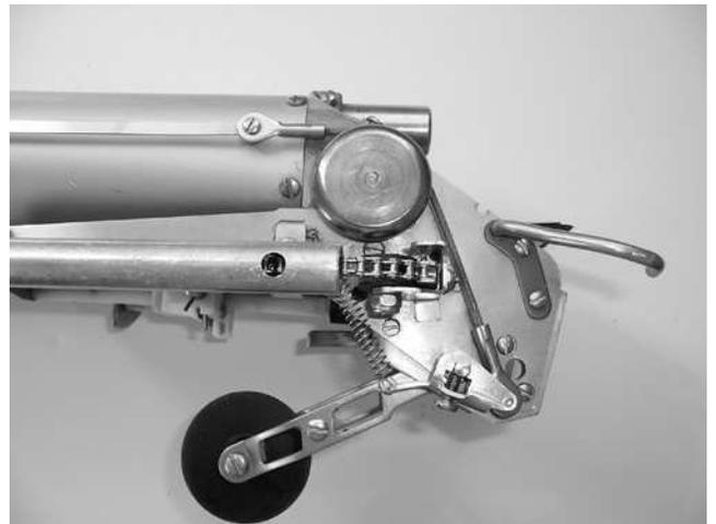
5) Remove pulley and shaft.
