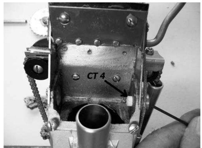
9) Use small screwdriver to push old CT 5 nyliner out of insert bushing.
