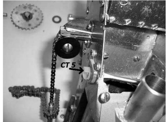
10) When installing new CT 5 nyliner, roll it in a circle and insert into bushing. Use small screwdriver to work ends together so it fits evenly in insert.
