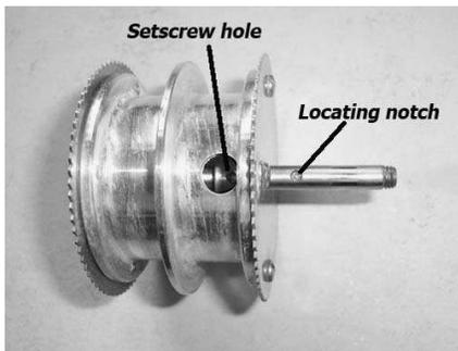
**Re-install drive drum on tape Tighten set screw**
