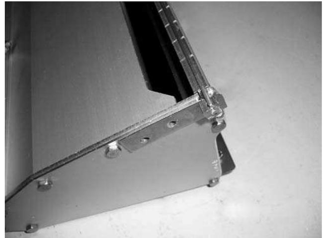
12) Install new shoe and adjust blade so it is .002" (or "thumbnail click") lower than blade. See diagram.
