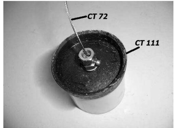
9) To replace cable, only the first retaining nut needs to be removed.
