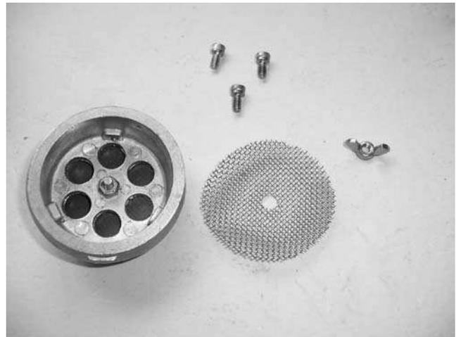
27) Use 5/16" wrench or nut driver to hold bolt on flapper valve side and 3/8" nut driver or wrench to remove lock nut on screen side.
