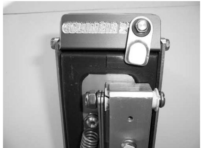
**\*\* Many people do not use the spring and the nail spotter will work without it. HOWEVER, with the spring on, it makes it easier to pull nail spotter cleanly away from wall or ceiling without leaving a tail of mud.**
