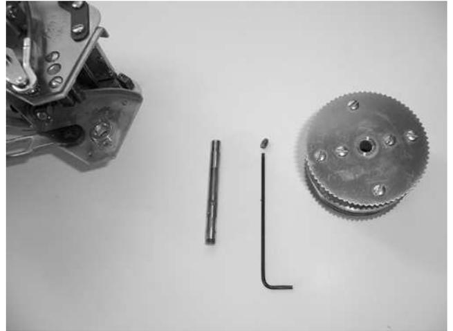
4) Turn mud shut off lever arm as shown to release cable guide pulley and clutch release shaft.
