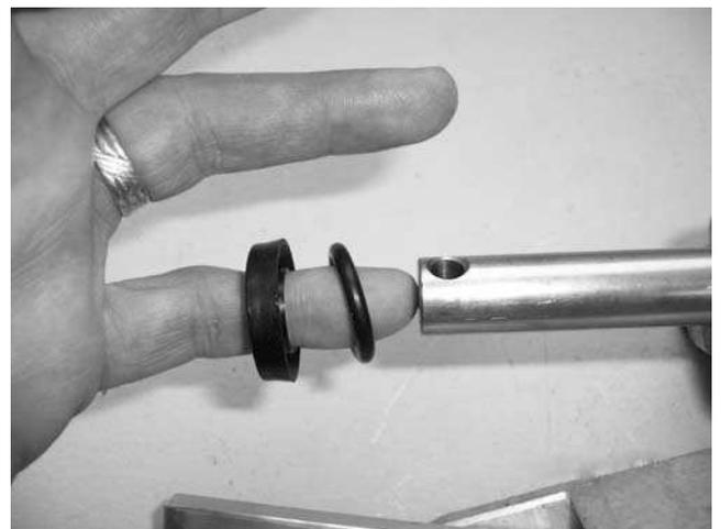
19) Slide seal and o-ring over shaft.
