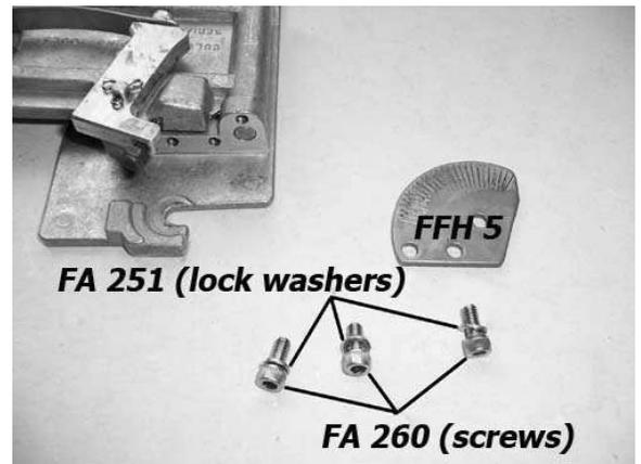
4) Replace with new friction brake disc and tighten three screws.
