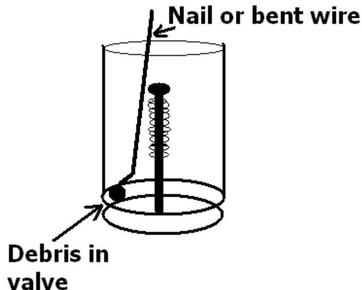
A small piece of uncoated copper wire or nail with a slight "L" bend at the end can be worked around the base of the valve housing to remove any debris lodged between housing and valve. After clearing around base of housing, flush again with water and the valve should no longer leak.
