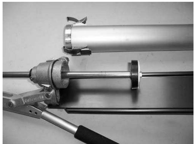
4) Cylinder and piston shaft off.
