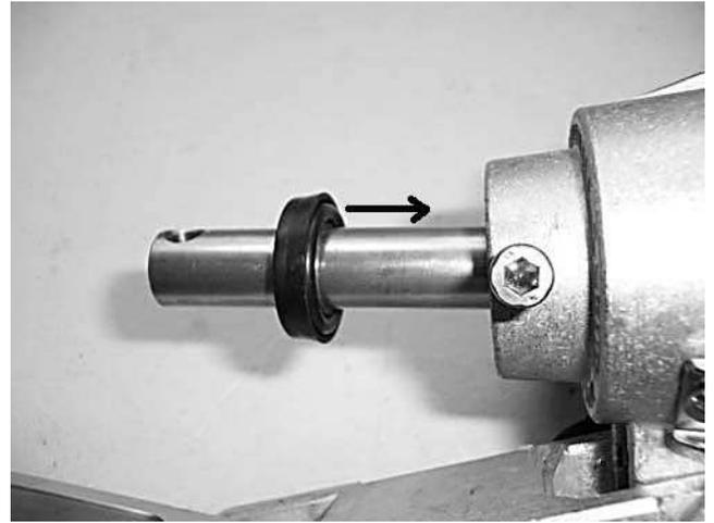
20) Seat seal and o-ring into head casting as shown.
