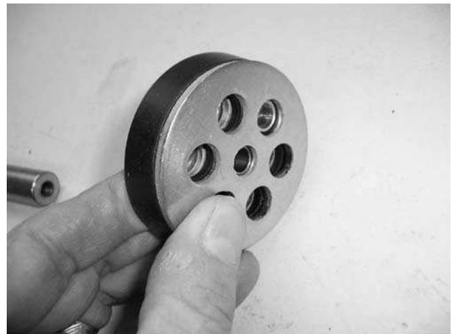
15) Hex bolt and washer in piston cup assembly.
