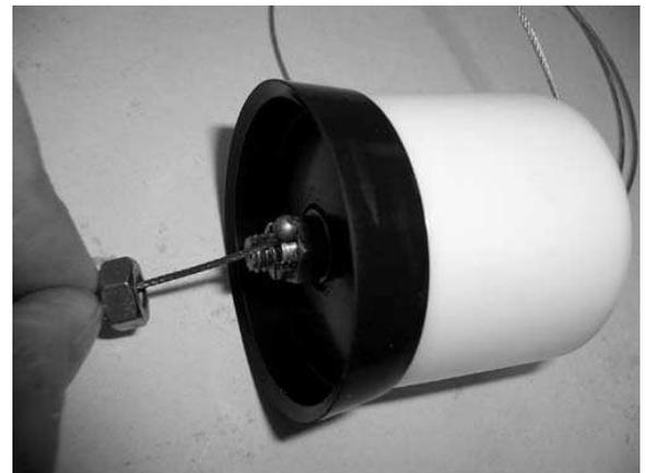
11) Insert piston back into taper tube and push in with wire at least half way up the tube.
