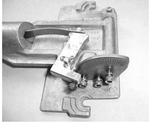
5) If the connecting strap FFH 9 breaks after long period of use, replace by first removing screw FA 260 from brass brake lever. This screw should also have a lock washer FA 251 to keep it tight.
