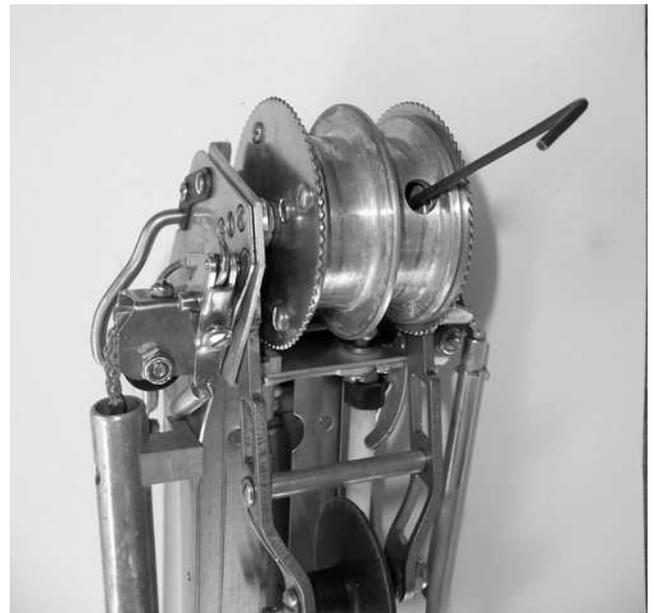
3) Drive drum and shaft removed.
