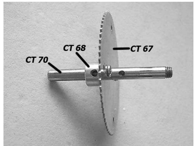
4) Attach both gear/hub assemblies to drum, tightening the screws a little at a time. Align with drive shaft. When gears are attached to drum, the assembly should spin freely on drive shaft. This is VERY IMPORTANT for easy re-assembly and future maintenance.
