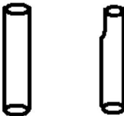
**Good bearing sleeve      Worn bearing sleeve**
