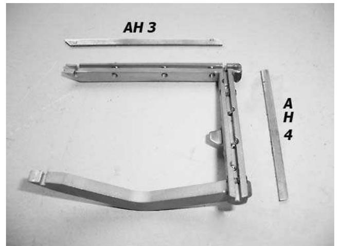
10) Before re-assembling, put frame on flat surface as shown (I use a small piece of granite tile, but a small piece of glass or mirror can work just as well.) Frame should not "rock" at either tip. If the frame does not rest perfectly flat, adjust tips a little at a time until frame no longer rocks at the tips.
