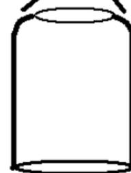
When the bearing sleeves become worn as shown, the roller may not track square in the corner. If your sleeves look like the worn version, they should be replaced.
