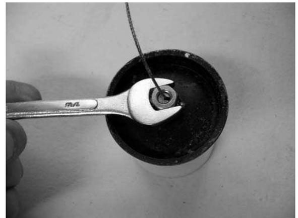
10) When attaching new cable, it should line up with groove in bolt and slot in special castle nut as shown.
