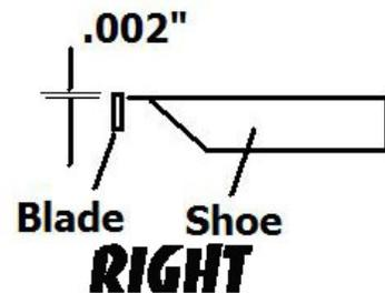
If the box blade is too much higher than the shoe, your box will leave "trails", in other words, the mud will finish to the sides of the seams, but box will leave a trail of mud on the sides of the finish.
