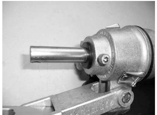
21) Slide shaft guide onto piston rod and push into head casting to seat seal.
