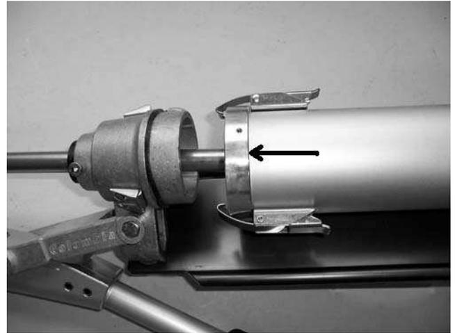
35) If you followed instructions, when the pump cylinder is clamped to pump head, thicker part of valve casting will be closest to pump leg as shown.\*\*
